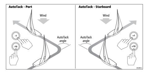
**Note:** If you have set the vessel type to SAIL BOAT, you can adjust the default AutoTack angle in User Calibration (see page 23).
